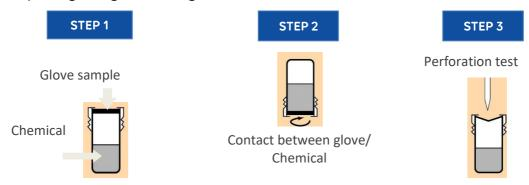
Deterioration (%) =  $(F0 - F1)/F0 \times 100$ F0: force of perforation without contact with the chemical F10: force of perforation after 1 hour of contact with the chemical
